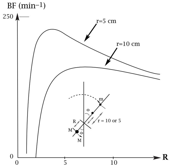
**Figure 1.** The beat frequency, BF, of a metronome as a function of the distance  $R$  of the heavy weight ( $M=40$  g) from the pivot axis at two fixed positions of the movable weight:  $r=5$  cm and  $r=10$  cm. As is evident, the beat frequency will be extremely sensitive to a small change in the position of the heavy weight—in particular for small values of  $r$ .
